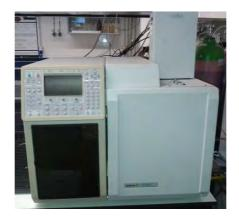
Figure 3.7 Picture of gas chromatograph (CP-3800)
