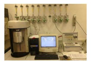
Figure 3.13 Picture of Micrometrics apparatus used to obtain nitrogen isotherms
