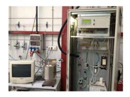
Figure 3.14 Picture of infrared adsorption analyser
