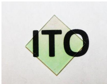
Figure 18. Image of the fabricated ITO substrate. Note its transparent optical properties.
