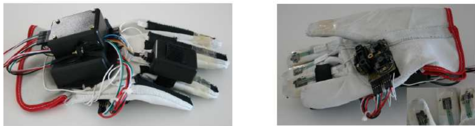
Fig. 1.5. Glove-based system prototype for measuring fruit attributes [57].
