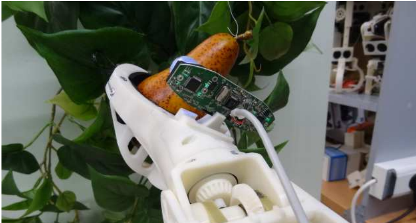
Fig. 5.1. Stereovision camera placed in the gripper of the robotic arm.
