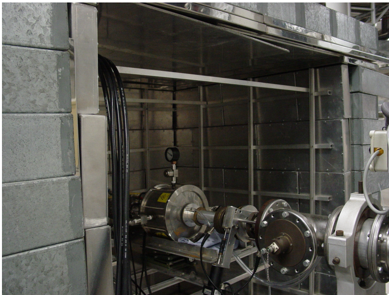
Figure 3.9: Picture of the beam line with the neutron producing target at the end, the TFGIC and the shielding structure around it.
