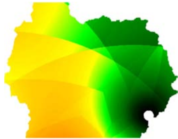
Fig. 1. Discontinuities in the resulting model caused by the moving neighborhood method.
