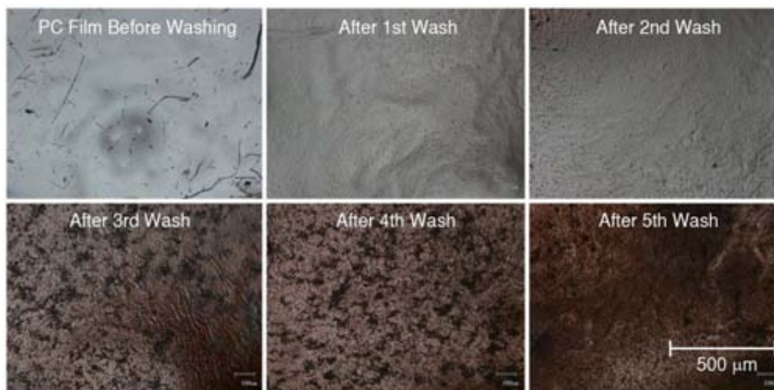
Figure 7-2. Photo images showing the gradual removal of the polycarbonate substrate of the pristine BL film by washing with \text{CH}_2\text{Cl}_2 . The the images were obtained using an optical microscope.
