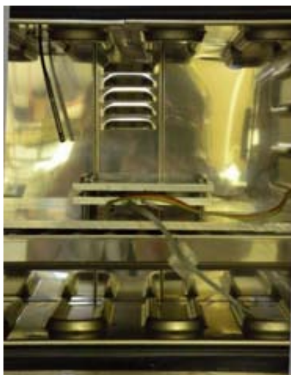
Figure 2-23. Image of the home-made sandwich-like device mounted within a Memmert chamber for controlled temperature annealing process.
