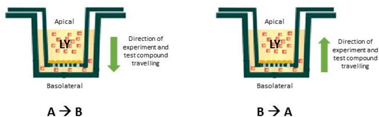
Figure 6.6. Illustration of experiments A \rightarrow B and B \rightarrow A in Caco-2 assay. In both experiments the Lucifer Yellow was added in the apical compartment, even though the antioxidant test solution addition was different. The test antioxidant travelled from the apical to basolateral compartment in experiment A \rightarrow B , and from the basolateral to apical compartment in experiment B \rightarrow A ; in contrast, LY travelled from A \rightarrow B in both experiments.
