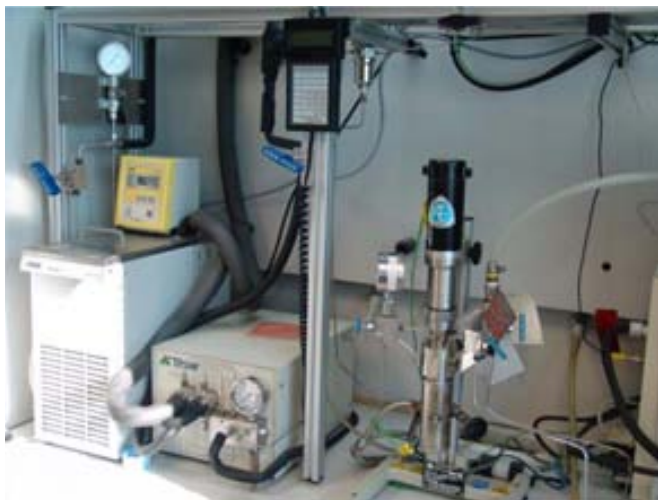
Figure 7.2. High-pressure equipment used for cations impregnation.
