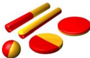
Figure 5.16. Schematic representation of some possible Janus particles. Red and yellow colors represent the different domains. 38
