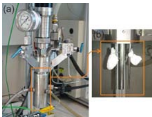
Figure 3.2. (a) 100 mL supercritical reactor used for the organic cations impregnation, and (b) paper packets containing the matrices hung from the thermobar.
