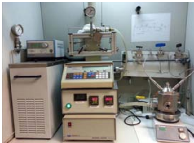
Figure 7.3. High-pressure equipment used for drug impregnation.
