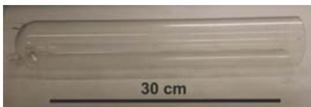
Figure 2.11. Pyrex vessel for the synthesis of aerogel-like silica particles, in which the sol is introduced inside the supercritical reactor.
