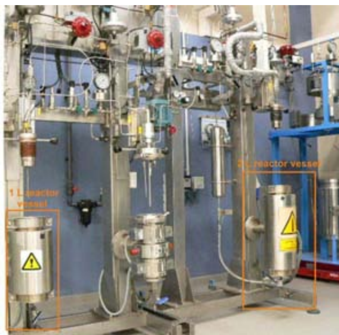
Figure 7.1. Pilot plant at MATGAS 2000 AIE used for the synthesis of silica-based materials.
