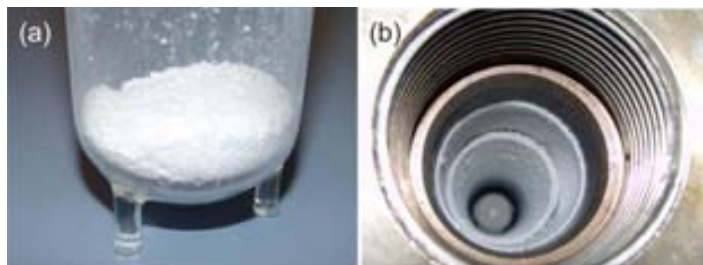
Figure 2.13. Photographs of aerogel particles: (a) sample inside the Pyrex vessel, and (b) the reactor just opened.
