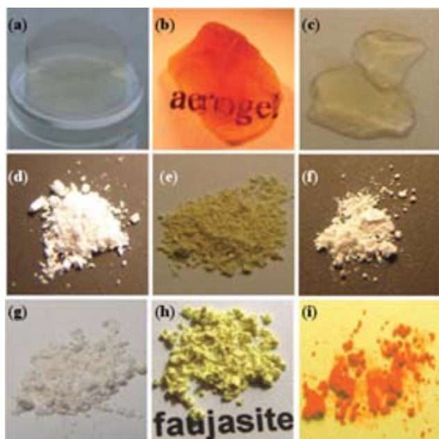
Fig. 2 Optical photographs of: (a) pristine monolithic aerogel (AM), and impregnated samples (b) [\text{Py}^+@AM] and (c) [\text{C}^+@AM] ; (d) pristine aerogel particles (AP), and impregnated samples (e) [\text{Py}^+@AP]_{sc} and (f) [\text{C}^+@AP] ; and (g) pristine zeolite Y, and impregnated samples (h) [\text{Py}^+@ZY]_{sc} and (i) [\text{C}^+@ZY]_{sc} .
