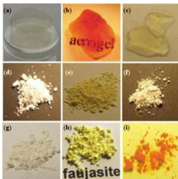
Figure 3.5. Optical images of: (a) pristine monolithic aerogel (AM), and impregnated samples (b) Py + @AM and (c) C + @AM; (d) pristine aerogel particles (AP), and impregnated samples (e) [Py + @AP] sc and (f) C + @AP; and (g) pristine zeolite Y, and impregnated samples (h) [Py + @ZY] sc and (i) [C + @ZY] sc .
