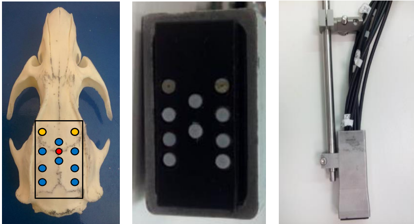
Figure 3.5: Left: Imaginary representation of the probe over the rat skull. Center: Overview of the surface probe. Right: Overview of the probe merged into the metallic shield.
