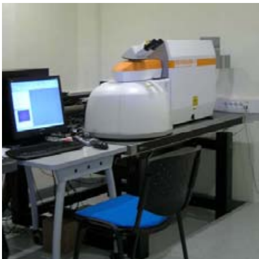
Fig. I. 10 Raman spectrometer Renishaw InVia from LASPEA Laboratory from the General Research Services (SGIker) of the University of the Basque Country (photography: K. Castro).
