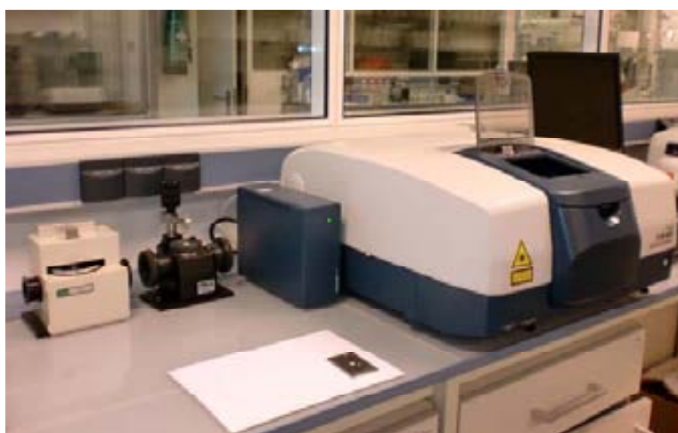
Fig. I. 13 JASCO 6000 Series FTIR (Japan) spectrometer of the IBea laboratory facilities at Parque Científico y Tecnológico de Bizkaia (photography: A. Pitarch).
