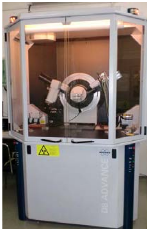
Fig. I. 8 Diffractometer D8 Advance (Bruker AXS GmbH, Germany) from the Service of X-Ray Diffraction of the ICTJA-CSIC (photography: A. Pitarch).
