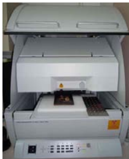
Fig. I. 7 Fisherscope® XDV-SD® (Helmut Fischer GmbH, Germany) spectrometer at the LARX facilities (ICTJA-CSIC) (photography: A. Pitarch).
