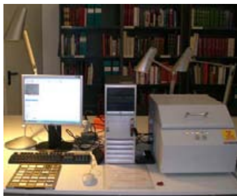
Fig. I. 6 Fisherscope® X-RAY XAN® (Helmut Fischer GmbH, Germany) spectrometer at the Numismatic Cabinet of Catalonia (GNC) facilities in the National Museum of Fine Arts of Catalonia (MNAC) (photography: A. Pitarch).
