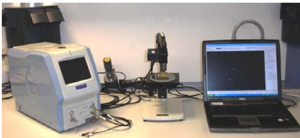
Fig. I. 9 Raman spectrometer innoRam ® (B&WTEK INC , Newark, USA) of the IBea 1 laboratory facilities at Parque Científico y Tecnológico de Bizkaia (photography: A. Pitarch).
