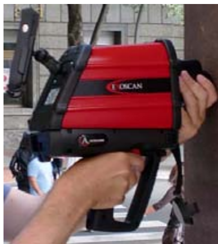
Fig. I. 11 Exoscan FTIR A 2 Technologies (Danbury, Connecticut, USA) spectrometer of the IBea laboratory facilities at Parque Científico y Tecnológico de Bizkaia (photography: A. Pitarch).
