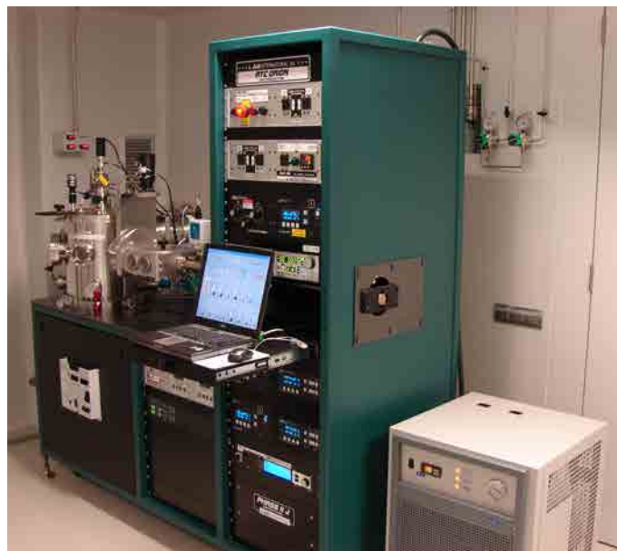
Figure 2.2: Picture of the ATC Orion 3 HV (top) and the ATC Orion 8 HV (bottom) installed in the Nanophotonics lab, ICFO.
