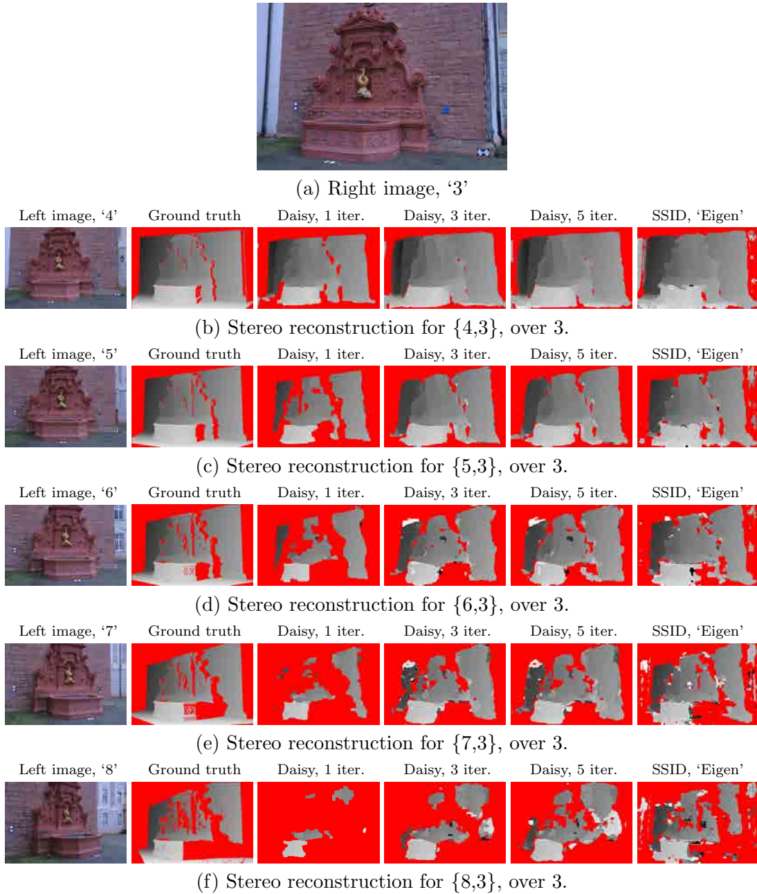
Figure 4.9: Qualitative comparison of the iterative stereo approach of Tola et al. (2010) with our segmentation-based, single-shot approach. We compute depth maps for image pairs \{x, 3\} , x \in [8, 4] , with an increasing baseline. All the reconstructions are over '3', the rightmost viewpoint, pictured in (a). (b-f): the first column shows the reference images; the second column the ground truth; columns 3-5 the Daisy reconstructions at iterations 1, 3, and 5; and the rightmost column the single-shot SSID-'Eigen' reconstruction. Occluded pixels are marked in red.
