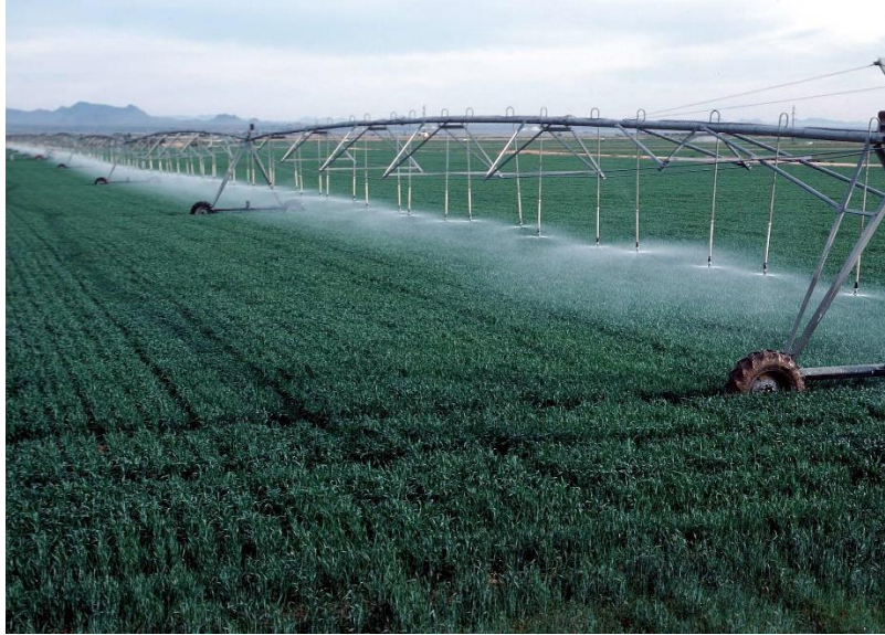
Figure 2.4: Center pivot with drop sprinklers.
