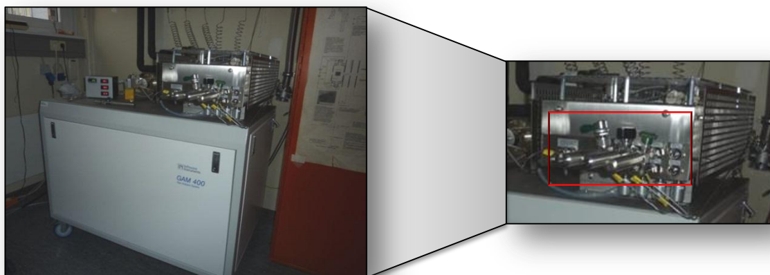
Figure. 3.3. Metallic gas sampling device connected directly to the gas mass spectrometer.
