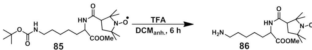
Scheme 6.11: Selective BOC deprotection of the PROXYL-Lys(BOC)-OMe radical ( 85 ) to obtain PROXYL-Lys-OMe ( 86 ).
