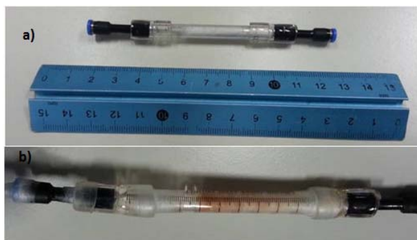
Figure 5.11: Filter used in the transfer process from the DNP to the NMR system to remove the radical from the hyperpolarized solution. a) Filter without using and b) filter after the transfer process. The orange color of the retained radical can be seen at the beginning of the filter.
