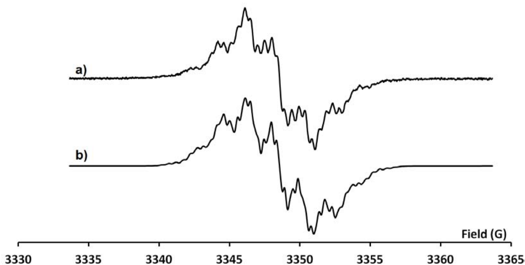
Figure 4.7: EPR spectrum of BDPA=BDPA diradical ( 42 ) at 300 K in THF/benzene. a) Experimental and b) simulated.
