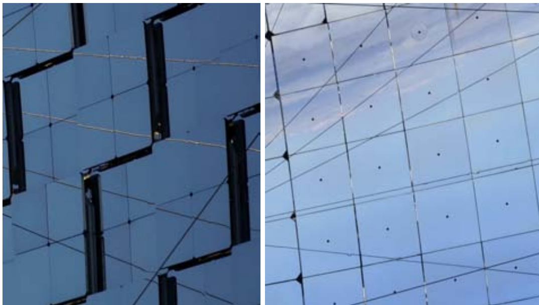
(a) MAGIC-I mirrors, each 1 m 2 unit is composed of 4 mirrors
