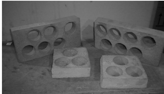
Figure 4.1 Sample extraction pattern: full bricks and half bricks obtained from flexural test.
