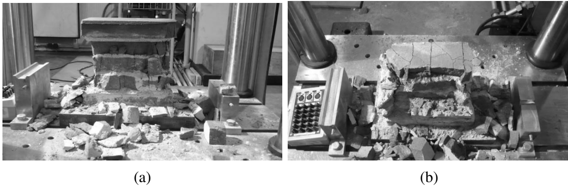
Figure 4.13 ALM prisms after testing: (a) with sulfur mortar cap and (b) with neoprene sheet.
