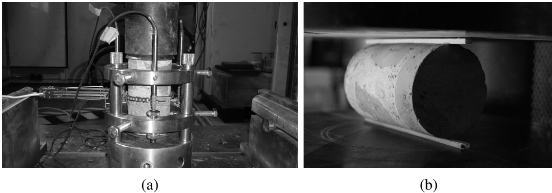
Figure 8.16 Test setup for infill testing: (a) compression test and (b) splitting test.
