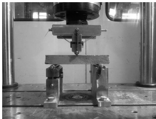
Figure 4.2 Brick flexural test setup.
