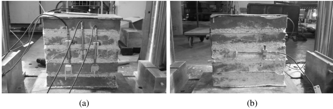
Figure 4.6 Typical layout of LVDTs: (a) vertical layout for displacement measurement in the unit and the composite and (b) horizontal displacement for measurement of the Poisson's ratio.
