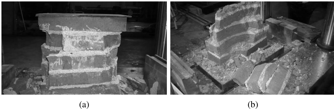
Figure 4.15 HLM prisms after testing: (a) with sulfur mortar cap and (b) with neoprene sheet.
