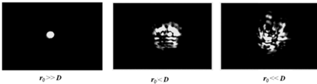
Fig. 3-2. Instantaneous image of a point source at the receiver plane under different turbulent scenarios depending on the Fried's parameter r_0 and the receiver telescope diameter D .
