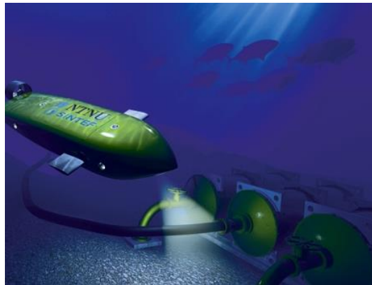
Figure 2.6: Munin AUV by NTNU/SINTEF. Inspection of pipelines and platforms
