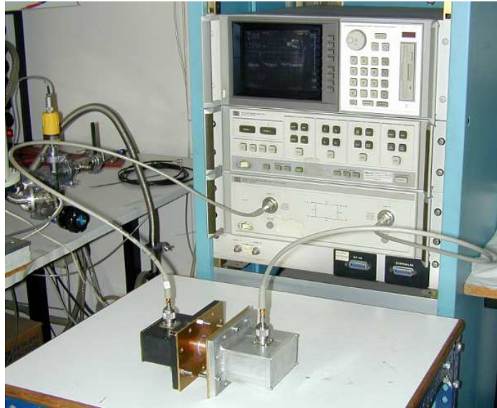
(c) Complete measurement setup including the HP8510C network analyser
