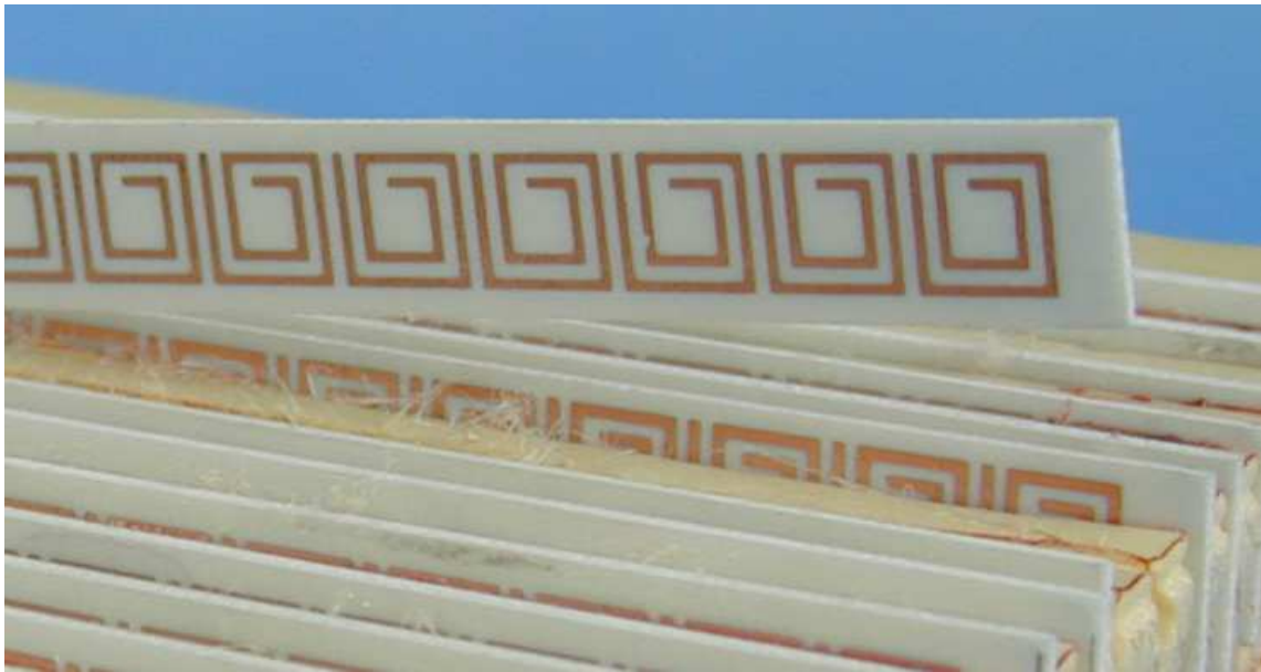
Figure 4.8: Fabricated single layer SR AMC on a Styrofoam board.
