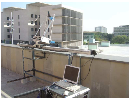
(a) GB-SAR system (top view)
