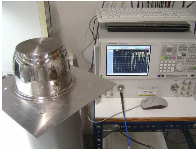
Figure 6.38: Measurement of the radiation efficiency with a Wheeler cap using an Agilent E8362B VNA.
