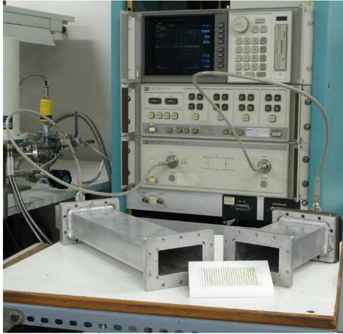
Figure 4.10: Open waveguide setup for S-parameter measurement.
