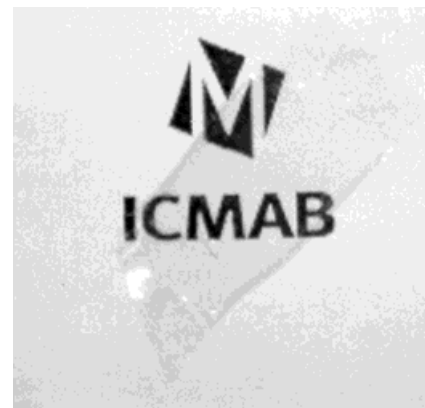
Fig. 2. View through the new metal-like BL film with a surface layer of \theta -(BET-TTF) _2 Br·3H _2 O nanocrystals (sample 6).
