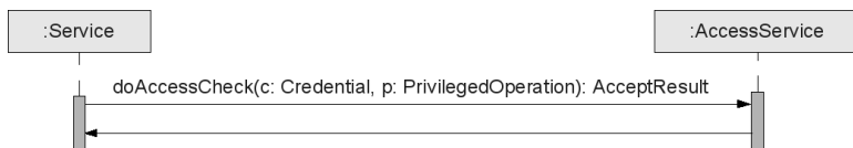
Figure 5.2: Access control check via Access Service
