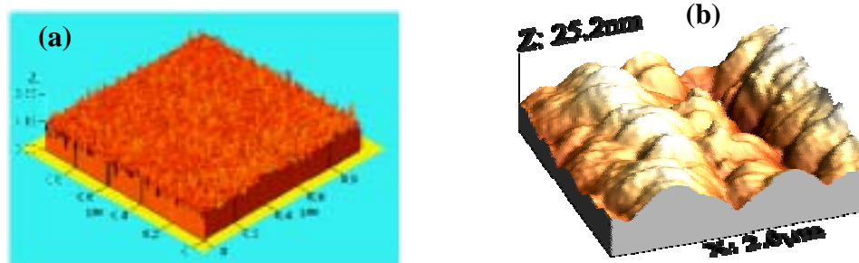
Figs. 3.1(a,b): (a) AFM analysis by 1 \cdot 1 \mu\text{m} scan of YSZ single crystal. (b) 2 \cdot 2 \mu\text{m} scan of YSZ(IBAD)/SS tape.
