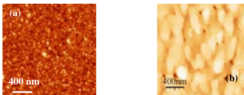
Fig. 4.3(a,b) : (a) AFM image of a standard sample of 25-30 nm thick CeO 2 grown at 750°C for 4 hours. (b) is the same sample but after a post annealing at 1000°C in static air[5].
