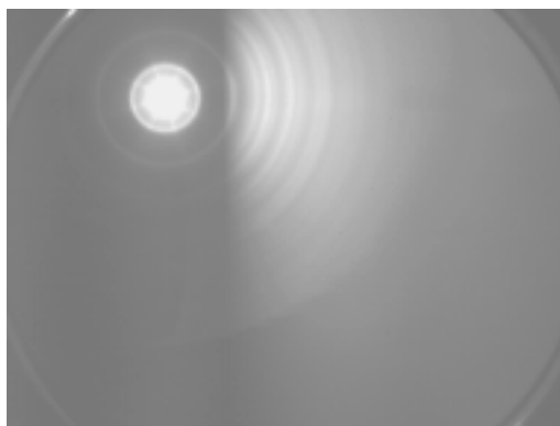
Fig 3.29: RHEED pattern of a CeO 2 film grown on YSZ at 750°C in Ar/H 2 exhibiting diffraction rings characteristic of a randomly oriented surface.
