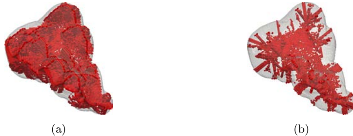
Figure 1.7: Medial surfaces obtained using a 6-connected neighborhood, (a), and a 26 connected neighborhood, (b).
