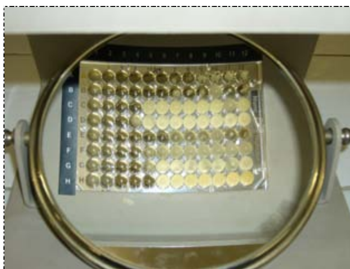
Fig. 24. Growth (turbidity) occurs in those wells with biocide concentrations below the MIC. Column number 12 was the negative control ( i.e. inoculated medium in absence of biocide).
