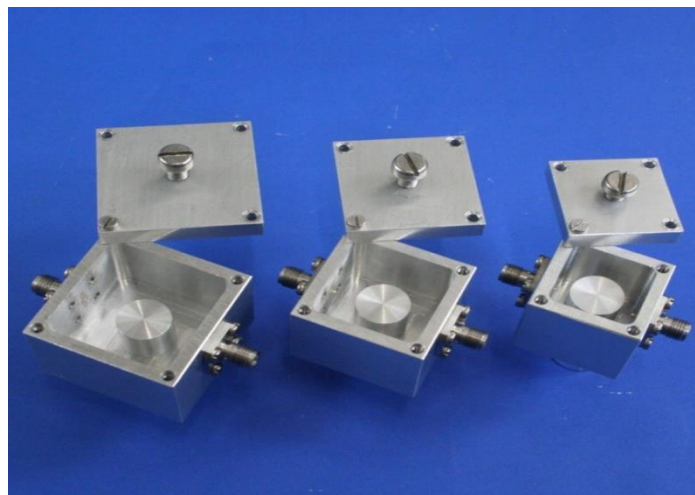
Fig. 95: Combine cavities fabricated for Q tests.
