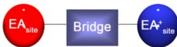
Figure 1.1. General representation of a MV system characterised by two electro-active-sites ( EA_{\text{site}} ) linked by a bridge that allows the electron transfer.
