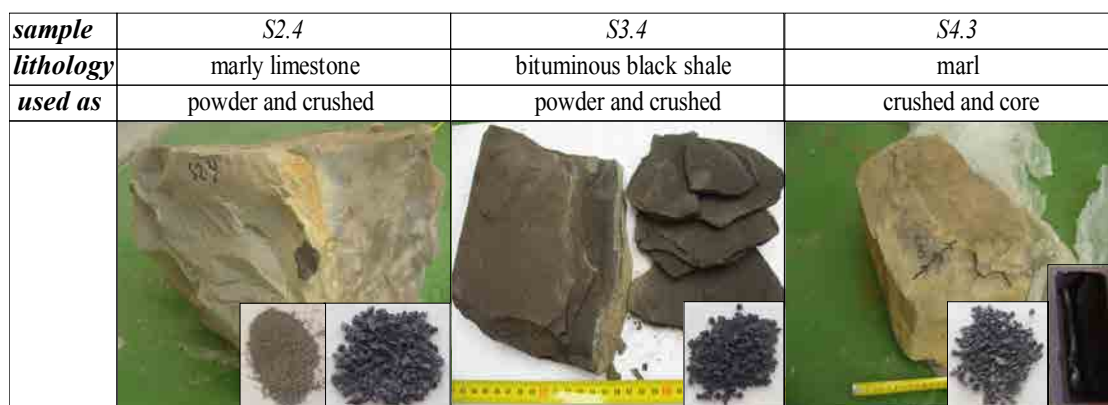
Figure 2.1 Picture of caprock samples from the Hontomín reservoir: marly limestone, bituminous black shale and marl. Inset images show powder (< 63 μm), crushed sample (1-2 μm) and core (18 mm in length and 9 mm in diameter).
