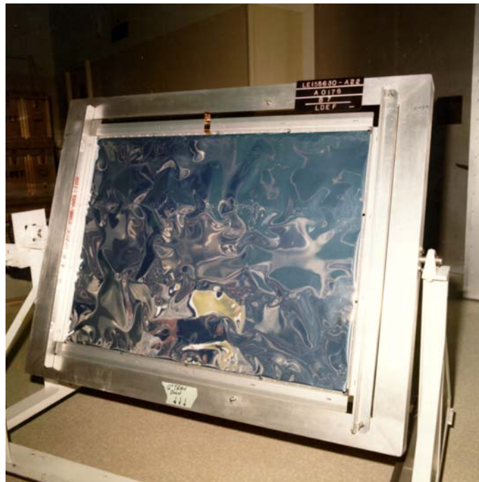
Figure 1.14. Final aspect of a tray of the UHCRE experince once mounted and before to be boarded on LDEF.
