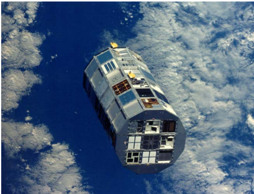
Figure 1.15. Picture of the LDEF satellite with the 76 trays containing all experiments, before to be launched in terrestrial orbit by means of the Challenger spacial shuttle.
