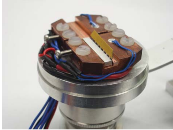
Figure 5.8: A custom double-oven, manufactured by qutools GmbH, allowed for separate temperature control of the ppKTP crystals. Foto courtesy of Pavel Trojek, qutools GmbH.
