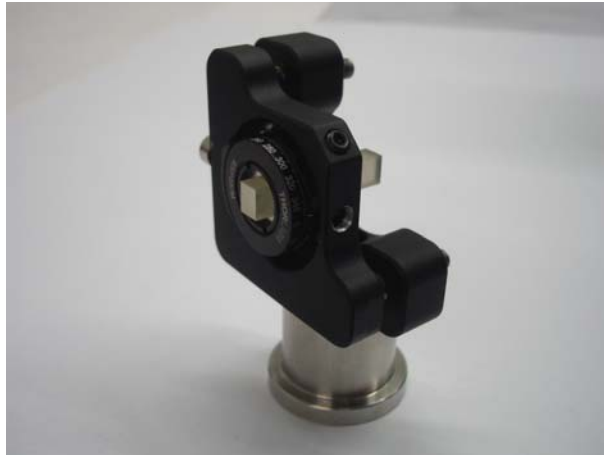
Figure 5.11: Custom-made miniature mount for \text{YVO}_4 compensation crystal. Foto courtesy of Pavel Trojek, qutools GmbH.
