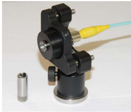
Figure 5.4: Custom-made miniature output coupler with adjustable focus, manufactured by qutools GmbH. The distance between the aspheric lens and the fiber tip could be adjusted using a spanner wrench (bottom left).
