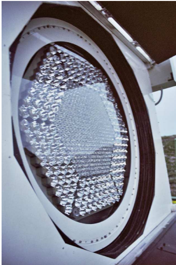
Figure 5.10: Front view of the MAGIC Telescope camera. The plexiglas window protects the camera interior where the light concentrators collect the incident light onto the camera photosensors.
