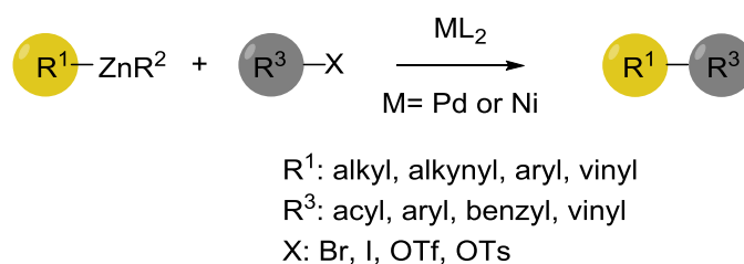
Figure 3.2.23 Negishi cross-coupling reaction. Image taken from Heravi et al. 327
