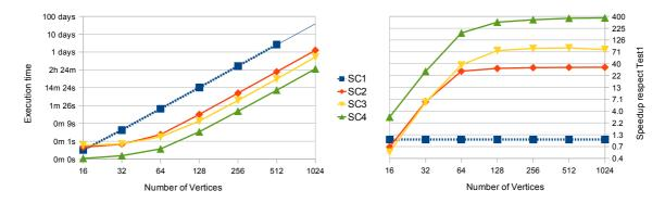
**Figure 6.15**: Run time of the 4 scalability tests respect to the number of vertices and speed-up of the parallel solutions (SC2, SC3, SC4) respect to the serial solution (SC1). Both plots vertical axis are in logarithmic scale.
