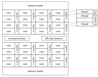
Figure 3.5: Overview of the BlueGene/Cyclops processor architecture.
