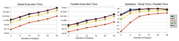
**Figure 6.18:** GREC run time of Serial and Parallel and speedup respect to the number of graphs for each selected class. Vertical axis are in log. scale.
