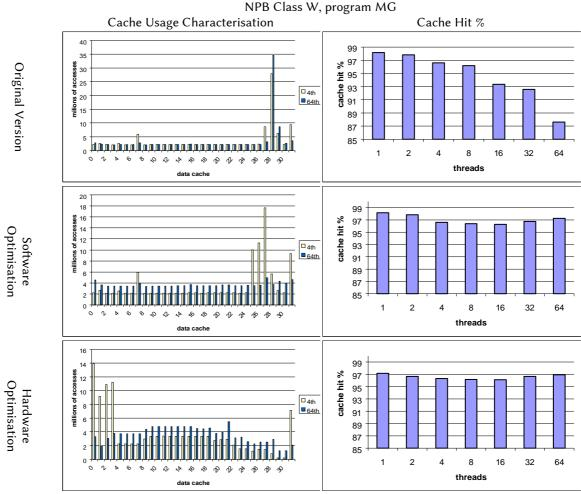
Figure 6.1: Cache behaviour for the MG Class W program in the IBM BlueGene/Cyclops architecture.
