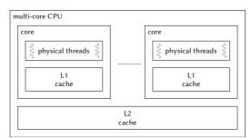
Figure 3.10: Overview of a desktop computer multi-core CPU.
