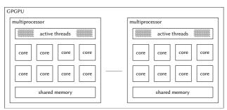
Figure 3.11: NVIDIA GPGPU architecture overview.
