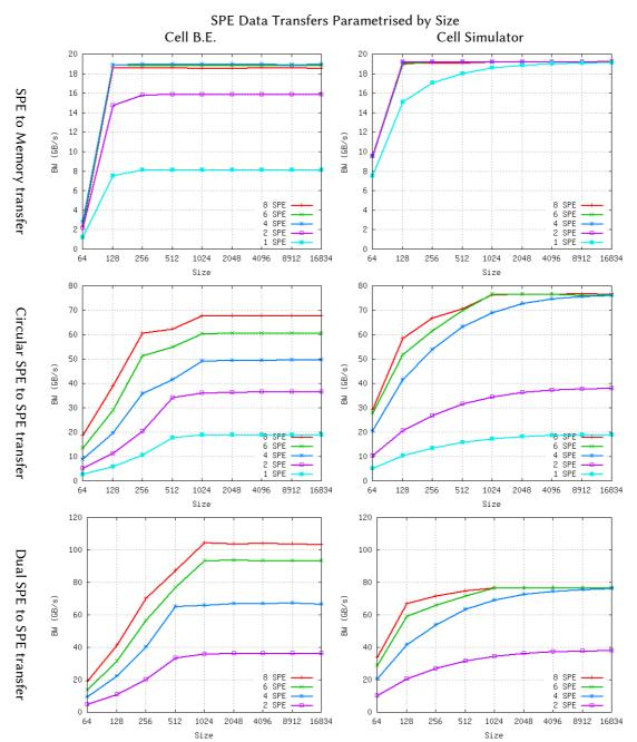
Figure 6.9: Cell B.E. versus Cell Sim SPE interconnection bus behaviour study.
