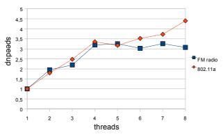
**Figure 6.10**: Stream programming model prototype scalability of FMradio and Nokia's Wifi 802.11a using only task and pipeline parallelism.
