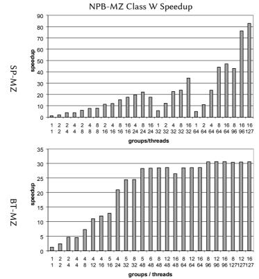
Figure 6.3: Scalability of the NPB-MZ programs class W in the IBM BlueGene/Cyclops.
