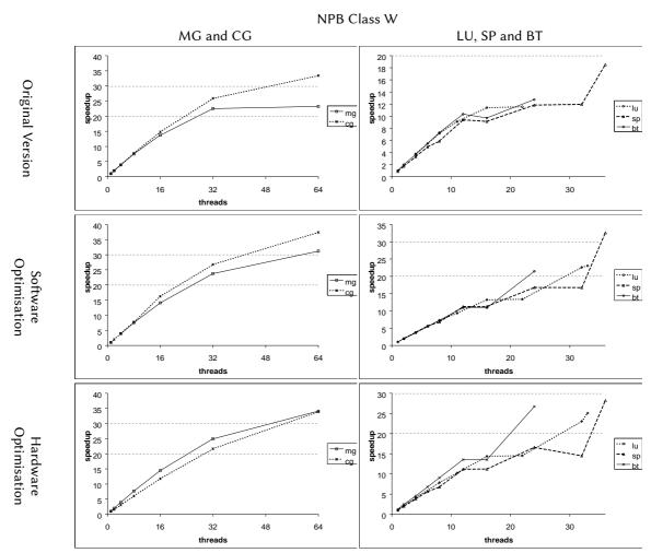
Figure 6.2: Scalability of the NPB programs Class W in the IBM BlueGene/Cyclops architecture.
