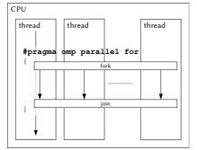
Figure 3.12: OpenMP fork/join thread execution model.
