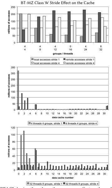
Figure 6.5: BT-MZ sharing threads on the same core effect on the cache of the IBM BlueGene/Cyclops.
