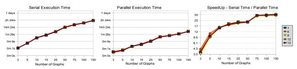
**Figure 6.17:** Letter run time of Serial and Parallel and speedup respect to the number of graphs for each selected class. Vertical axis are in log. scale.
