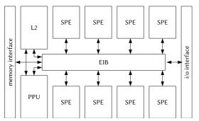
Figure 3.7: Cell B.E. Sony Playstation3 processor implementation block diagram.
