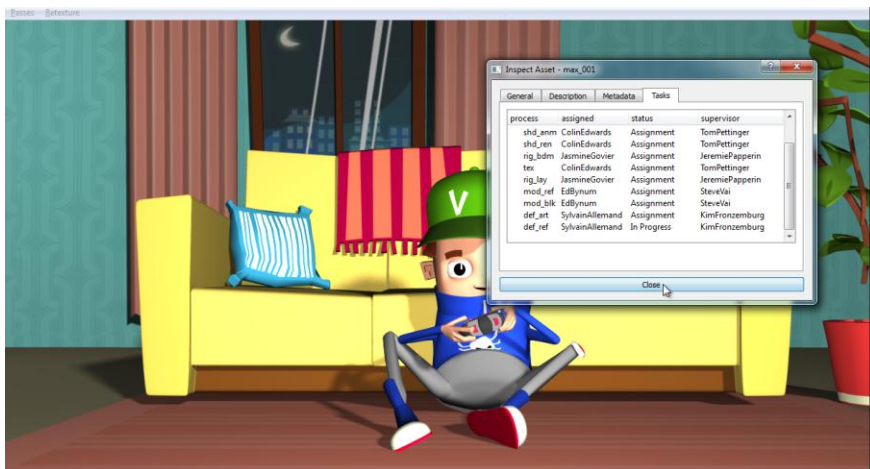
Figure 3.4.4: This figure shows a rendered frame from the shot, open in my prototype review tool. When clicking on a pixel, the tool extracts the code of the asset depicted in the selected pixel and retrieves all the relative production data from the DAMS and DPMS.
