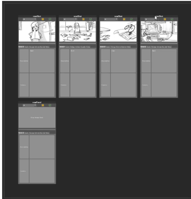
Figure 3.3.2: A complete sequence can be described as a set of panels. Each shot is described by one or multiple panels that contain all the relevant information for the pipeline and the artists. This information includes description of the shot, camera description, the list of assets, sounds, actions and dialogues. The panel also shows the status and the feedback for the shot.
