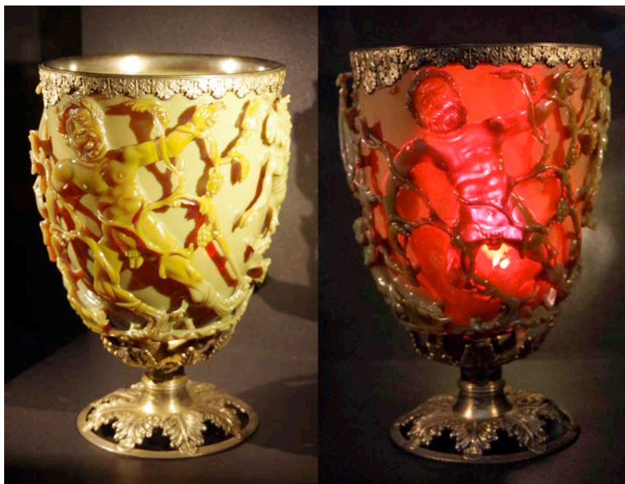
Figure 10 – The Lycurgus Cup, at the British Museum of London, coloured in green in reflected light (left) and coloured in red in transmitted light (right). These two colours are due to the presence of gold and silver nanoparticles in the glass.
