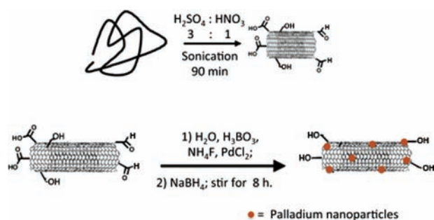
Figure 1. Scheme of the decoration of the multi-walled carbon nanotubes. (a) Surface functionalization of the MWCNTs; (b) In-situ synthesis of the palladium nanoparticles on the surface of the functionalized MWCNTs.
