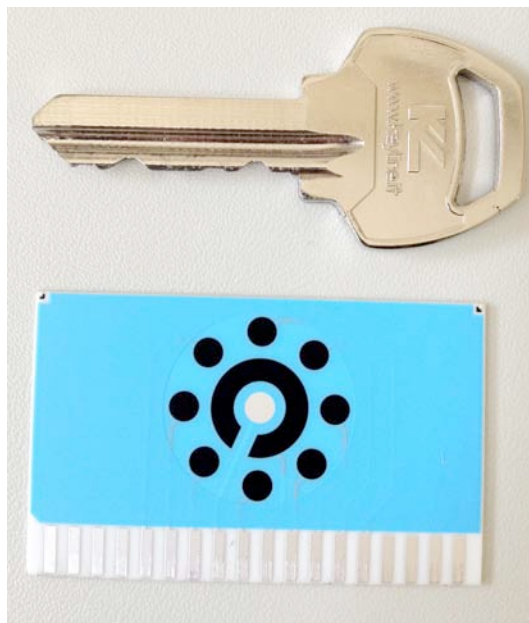
Figure 5.1 – Custom screen-printed multi electrode, the black outer circles are eight working electrodes, the quasi-complete black circle in the middle is the auxiliary electrode and the small silver circle in the middle is the pseudo-reference electrode; a normal key is showed to size comparison.
