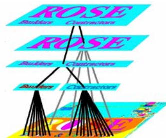
Figure 5.1: A natural scene image and a hierarchical representation of its text. Atomic objects (characters) extracted in the bottom layer are agglomerated into text groupings at different levels of the hierarchy.
