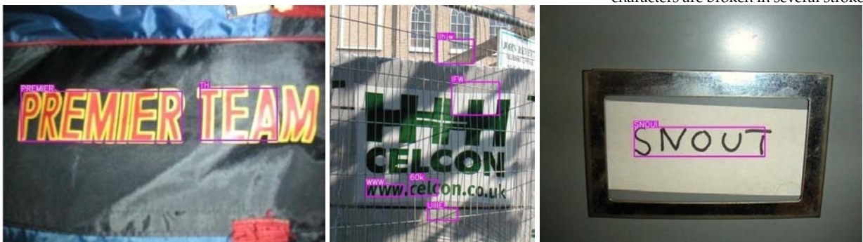
Figure 9.5: Common errors when segmentation is particularly challenging or characters are broken in several strokes.
