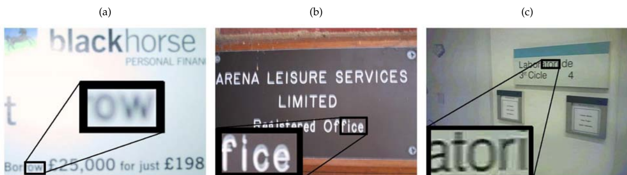
Figure 1.4: Examples of inherent challenges of digital camera imaging: (a) uneven focus, (b) motion blurring, (c) image compression artifacts.
