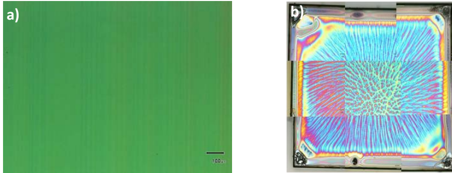
Figure 4.22. Optical microscope images of a) a pristine YBCO film and b) YBCO+6%M CeO 2 -TREG film after the pyrolysis process.
