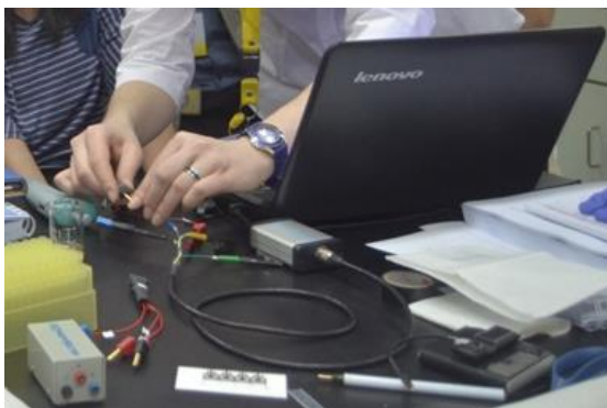
Figure 1.8 Representation of a miniaturised electrochemical device using screen-printed electrodes.
