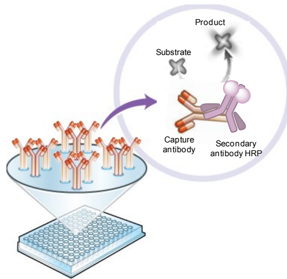
Figure 3.5 Schematic representation of the ELISA for the determination of the total antibody coupled on the modified MPs. (Adapted from Abcam website, www.abcam.com )
