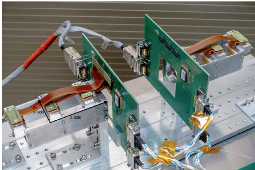
Figure 7.2: Photo of the AIDA SBM FE-I4 telescope. The two telescope arms are movable along the z and y axes.
