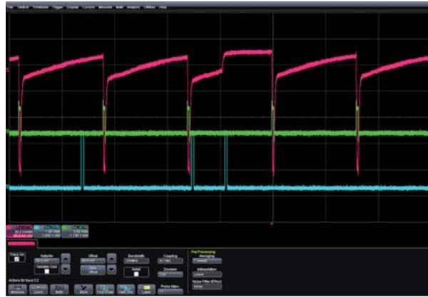
Figure 6.9: Analogue pixel signal of a 100\ \mu\text{m} \times 100\ \mu\text{m} pixel (in pink) exposed to 160 GeV pions. The change in slope after the passage of the MIP through the pixel indicates saturation.
