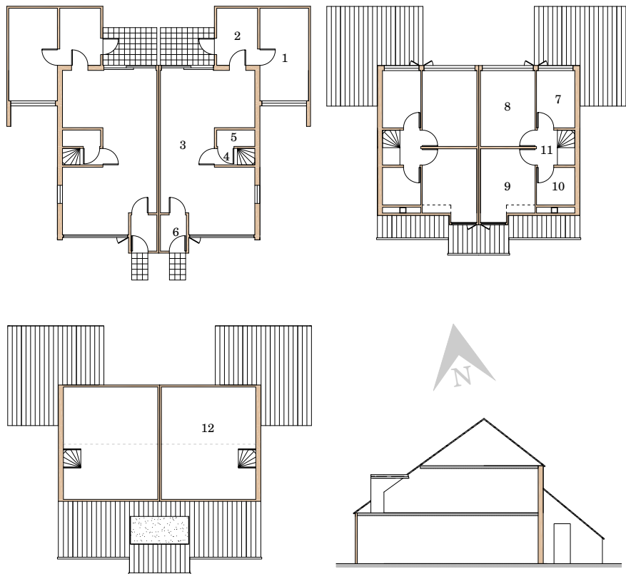
Figure 4.18: House drawings. From top to bottom and left to right: ground, first and attic front views and building lateral view. The drawing scale is 1:42.
