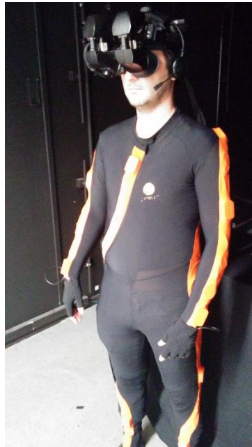
Figure 3.5: IVR setup. Body tracking Xsens suit, head tracking Intersense IS-900, NVIS nVisor SX111 HMD, and headphones with a built-in microphone.
