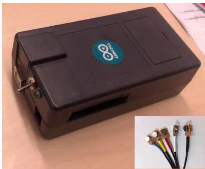
Figure 7.7: The Arduino Uno board enclosed in a box. On the bottom right, the vibrator devices.
