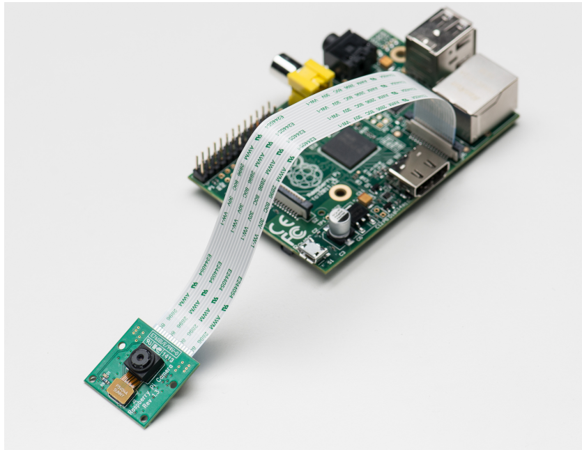
Figure 4.2: Raspberry Pi with an attached camera module. Image from Adafruit Industries (CC BY-NC-SA 2.0).
