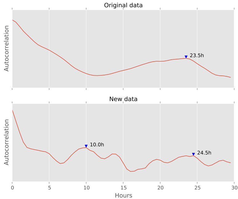
Figure 3.7: Detail of the autocorrelation for video a . A peak at \sim 24 hours indicates a circadian periodicity on the original data. Peaks at \sim 24 and \sim 12 hours on the new data indicate circadian and ultradian periodicities respectively.
