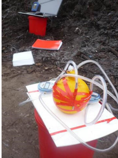
Figure 39: Our sensor with four probes attached to its surface with a 90^\circ
