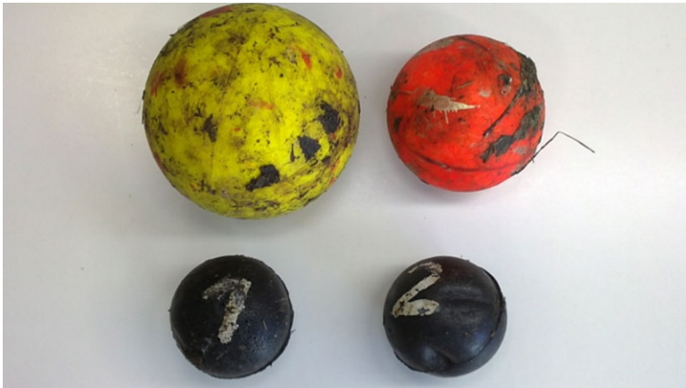
Figure 18: Capsules after the test in an urban composter
