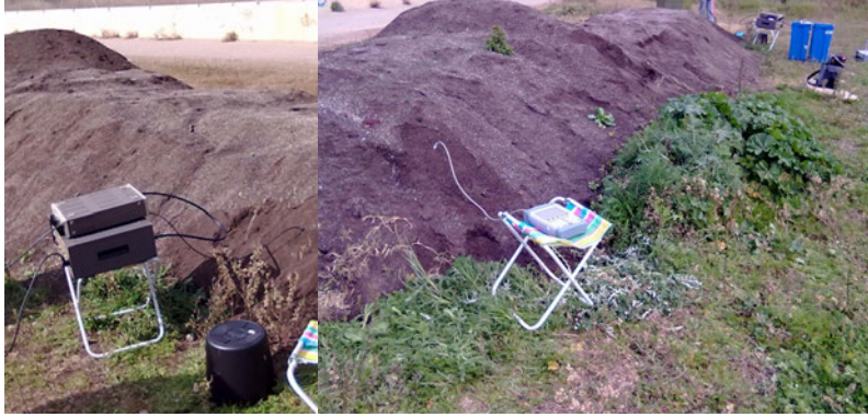
Figure 46: Experimental setup. (left) Signal generator and gain amplifier. (right) Spectrum analyzer.
