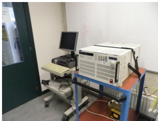
Fig. 2.5. Programmable load AMREL PLA7.5K-600-400 and simulation station
