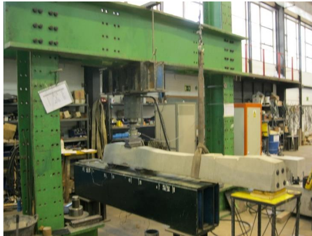
Fig. 3. Setup of the static positive load test at the rail-seat section [46].
