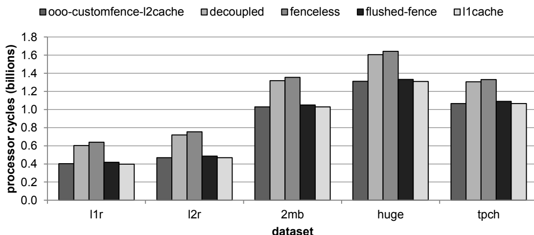
Figure 2.4: Hardware design space exploration running the vectorised hash join probe binary when MVL = 64 .
