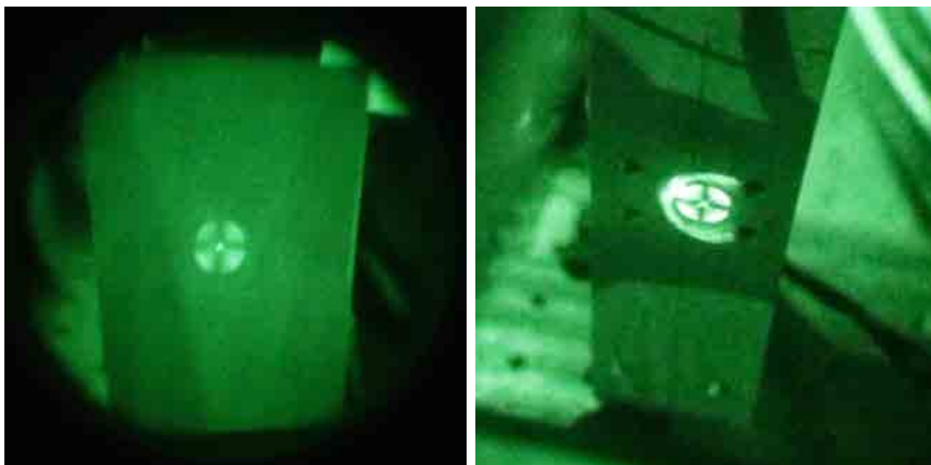
FIGURE A.3: The photographs are taken by placing an infra-red viewing camera in front of a smartphone camera.
