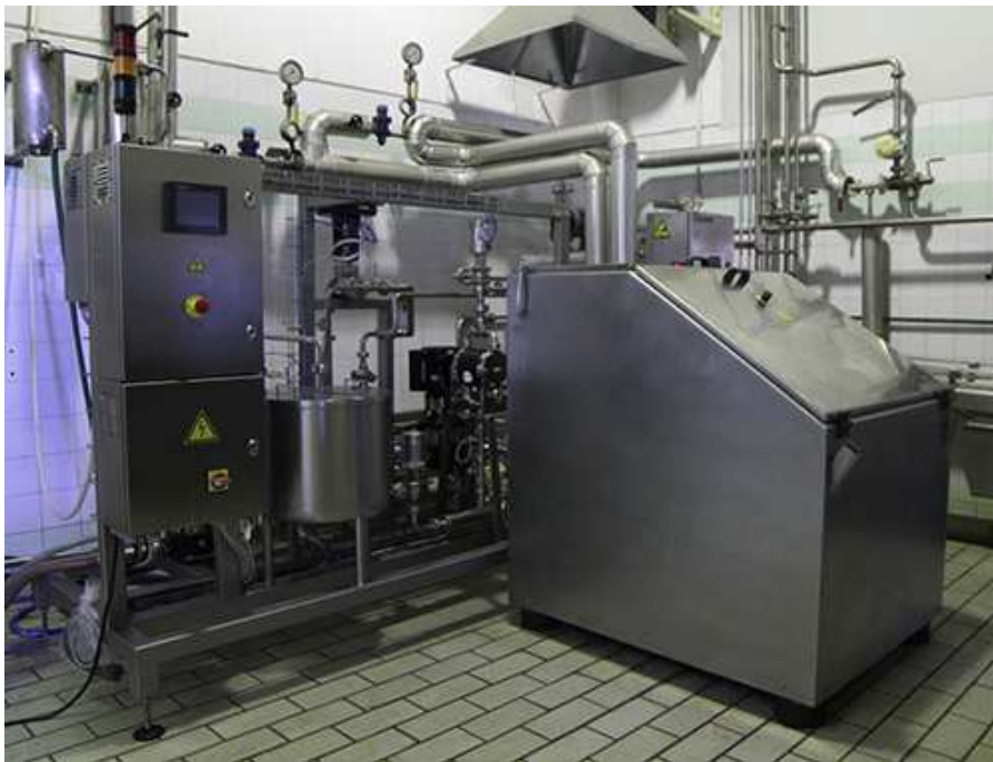
Figure 7. Ultra-High Pressure Homogenization system used in the present PhD thesis developed by Ypsicon SL, Barcelona, Spain.
