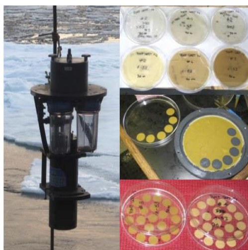
Figure 2.4: In situ pump being deployed (left image). On the right, Nitex screens used to collect the fraction >53\ \mu\text{m} (top), QMA filter used to collect the fraction 1\text{--}53\ \mu\text{m} with few 21\ \text{mm} punches removed from the main filter (middle) and the total 21\ \text{mm} diameter punches obtained from QMA filters (bottom).
