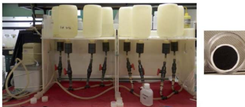
Figure 2.1: Filtration system with 8 bottles connected to an Eyela aspirator vacuum pump (left image) and the resulting QMA filter with \text{MnO}_2 precipitate (right image).
