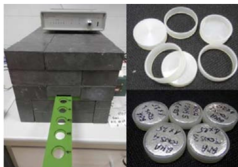
Figure 2.2: RISØ beta counter covered by a shield of old lead, with an anticoincidence module on top and the green filter support outside the detector (left image). On the right, empty plastic RISØ cups (top) and samples mounted on plastic RISØ cups ready to be measured (bottom).
