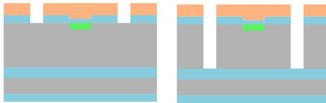
Figure 4.9: \text{SiO}_2 etching and DRIE to create the cylindrical annulus.
