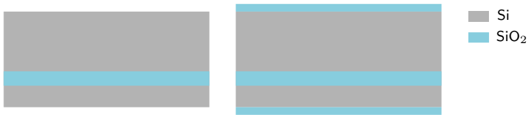
Figure 3.9: SOI wafer and wet oxidation process.
