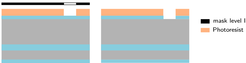
Figure 3.10: Photolithography process and SiO 2 etching.
